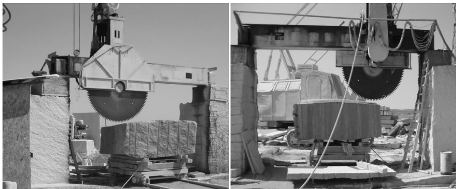
Fig. 1.1. The process of sawing a granite block with a diamond disc saw
